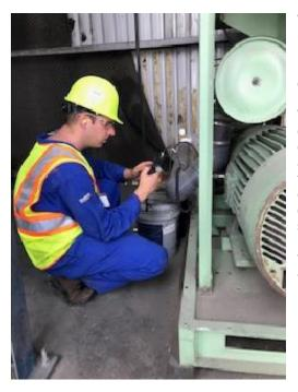
Vibration troubleshooting is routinely applied to rotating and reciprocating equipment to assess general mechanical health. Bearing, motor, gearbox, driveline and foundation problems can be easily identified prior to becoming an operational problem.
